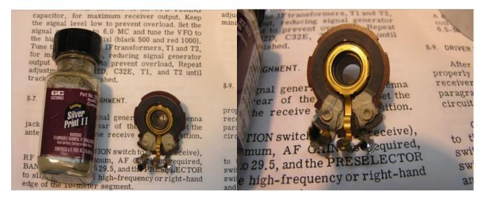
I believe the construction of the pot precludes any of the controls from reaching ideal 0 ohms and that the vast majority of rigs would benefit from some type of corrective action.
