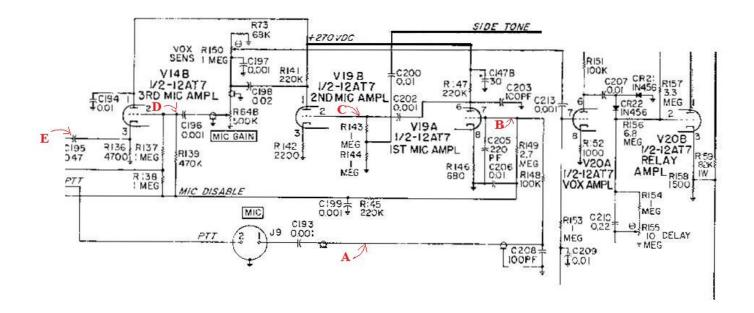
The mic amplifier is composed of one half of V14 and V19. V19 is operational at all time in all modes. V14B is biased on only when the transmitter is keyed in one of the SSB modes. For the following test you will need to inject a 1KHz signal from a 600 ohm source, into pin 1 of the mic jack. To measure the signal at test point E you will need to apply a ground to pin 2 of the mic jack.
