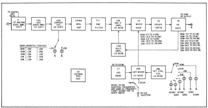
Figure 6. Block Diagram of Model HT-46 Transmitter.
