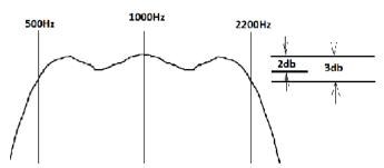
NOTE: If the bandpass is too narrow and you cannot broaden it adjusting L1 and L2 check the alignment of L3 and the value of R25 (22K). R25 is a swamping resistor used to lower the Q of L3 and widen its bandpass.
