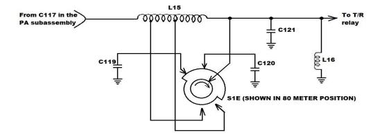
OK, let's attack C119, 120 and 121. Only C121 is used on 20-meters. C120 and C121 are both used on 40 meters. All three on 80. Therefore, we will start at 20-meters.
